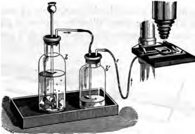
FIG. 39.—GAS CHAMBER IN USE WITH APPARATUS FOR GENERATING CARBONIC ACID.
